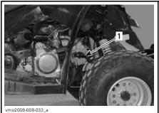
TYPICAL — RH SIDE OF VEHICLE 1. Spark plug location
